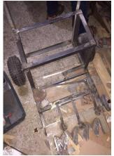
**Fig. 3** – Assembly of Frame, Cutter and Wheels
