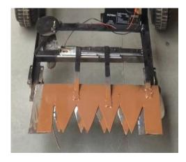
Fig. 2 – Cutter Blades and Slider Crank mechanism
